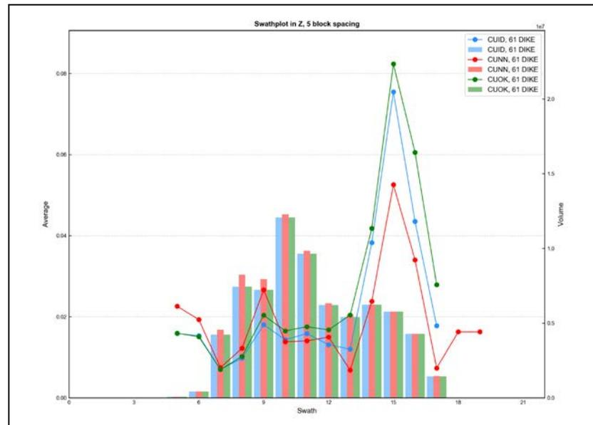
Figure E - 117 Swath Plot in the Z Direction of Total Copper for the Dikes
