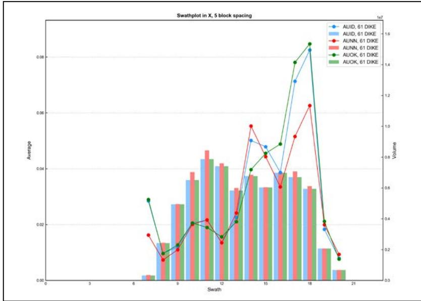
Figure E - 112 Swath Plot in the X Direction of Gold for the Dikes
