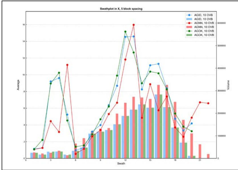
Figure E - 13 Swath Plot in the X Direction of Silver for the Overburden
