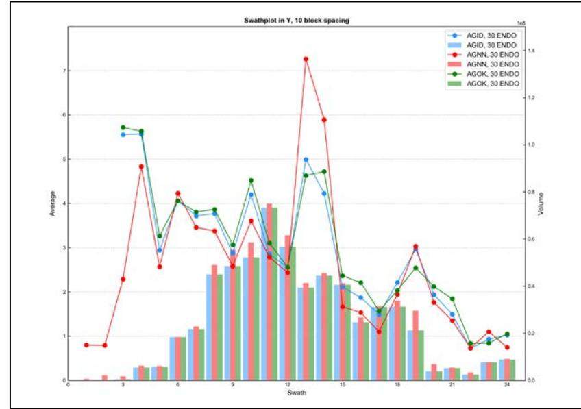
Figure E - 50 Swath Plot in the Y Direction of Silver for the Garnet Skarn
