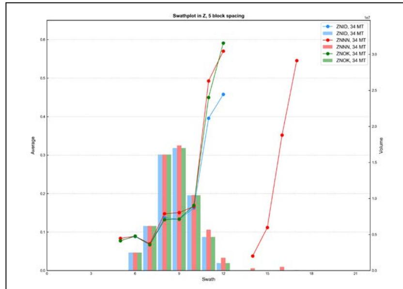
Figure E - 84 Swath Plot in the Z Direction of Total Zinc for the Magnetite Skarn
