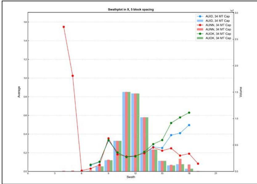
Figure E - 76 Swath Plot in the X Direction of Gold for the Magnetite Skarn
