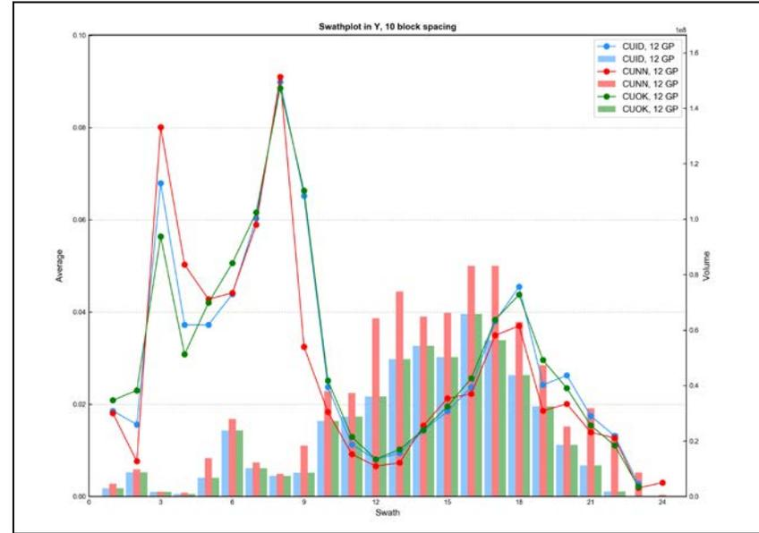
Figure E - 32 Swath Plot in the Y Direction of Total Copper for the Granite Porphyry
