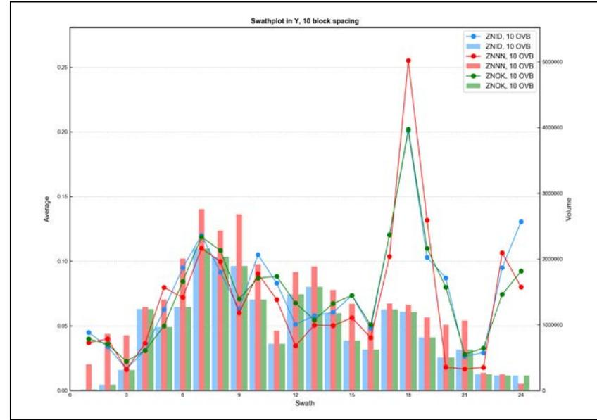
Figure E - 23 Swath Plot in the Y Direction of Total Zinc for the Overburden
