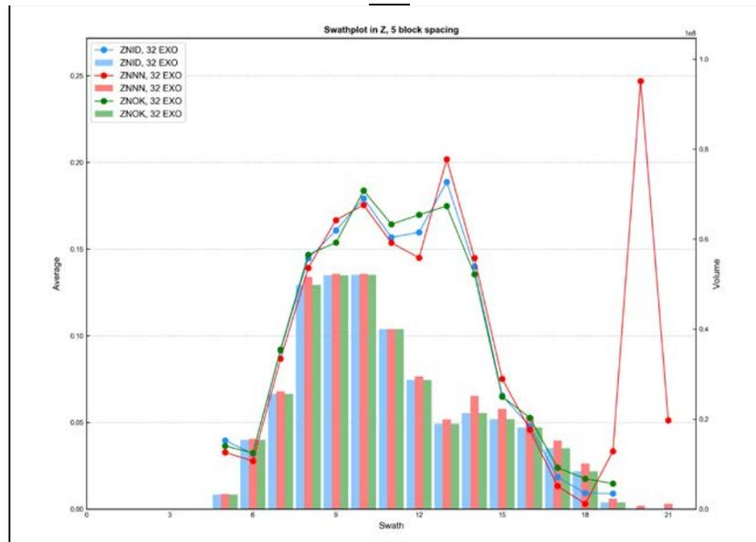
Figure E - 72 Swath Plot in the Z Direction of Total Zinc for the Pyroxene Skarn
