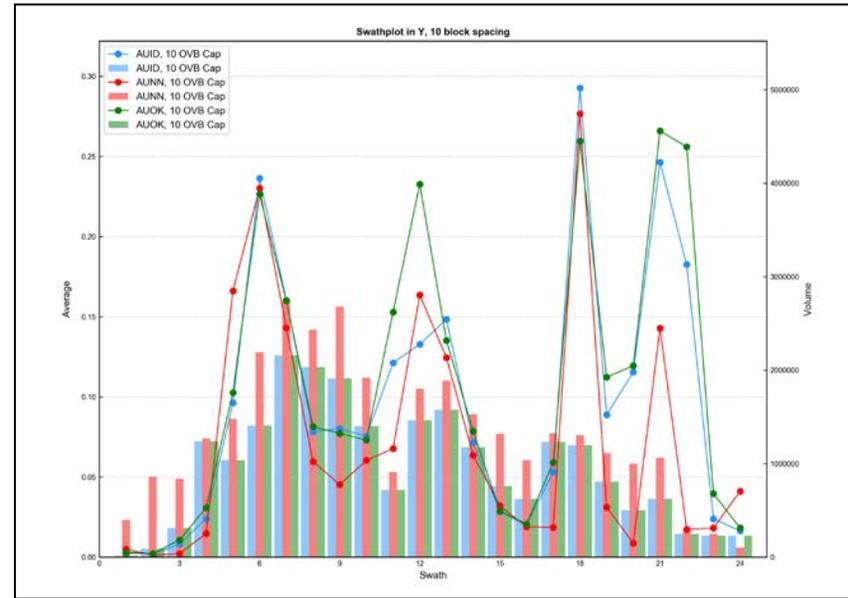
Figure E - 17 Swath Plot in the Y Direction of Gold for the Overburden
