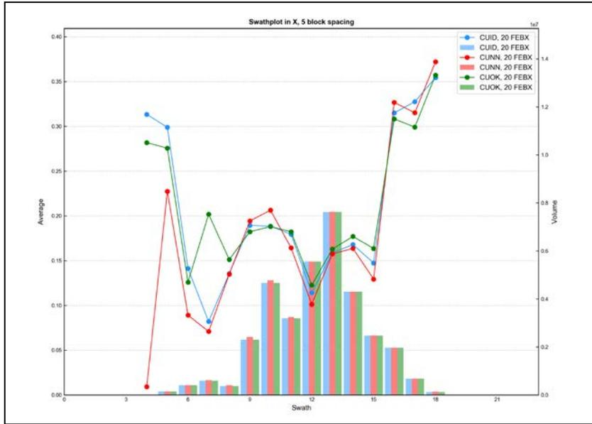
Figure E - 45 Swath Plot in the X Direction of Total Copper for the Iron Oxide Breccia
