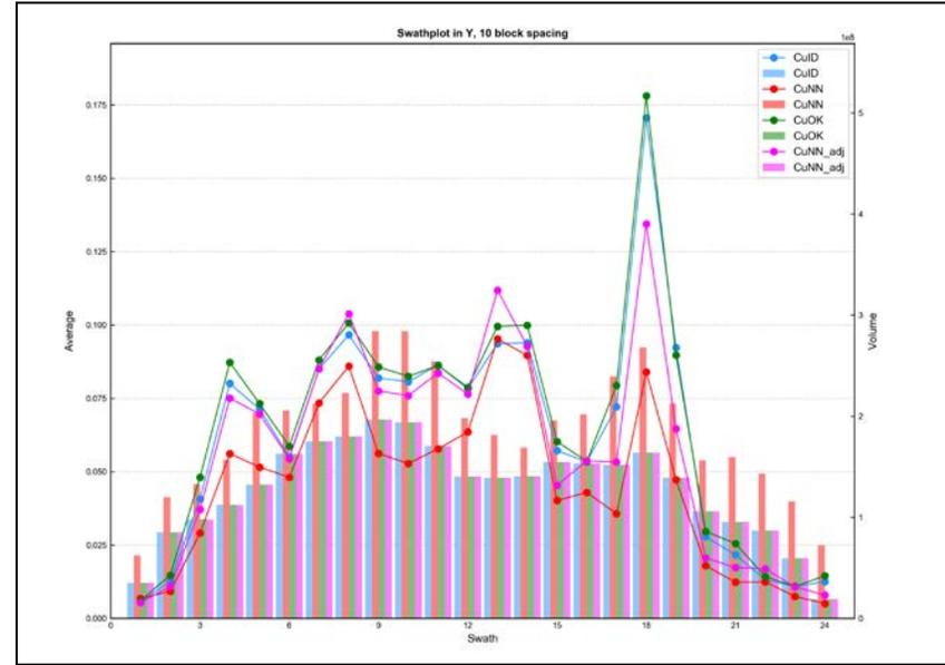
Figure E - 8 Swath Plot in the Y Direction of Total Copper for the Global Resource
