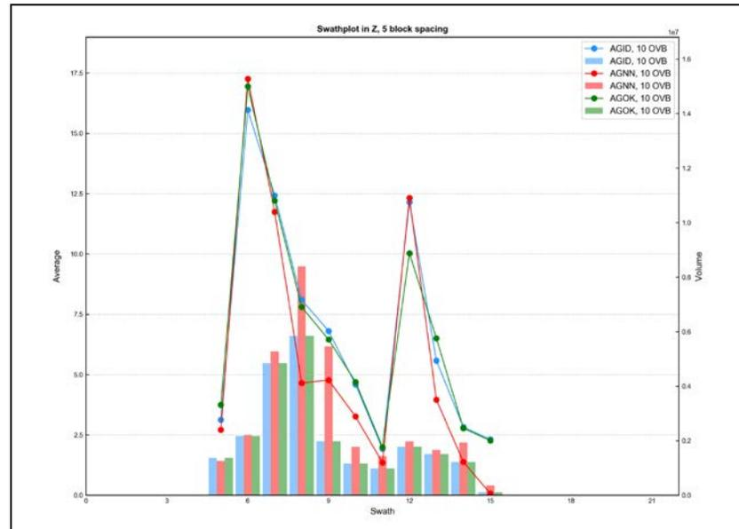
Figure E - 15 Swath Plot in the Z Direction of Silver for the Overburden
