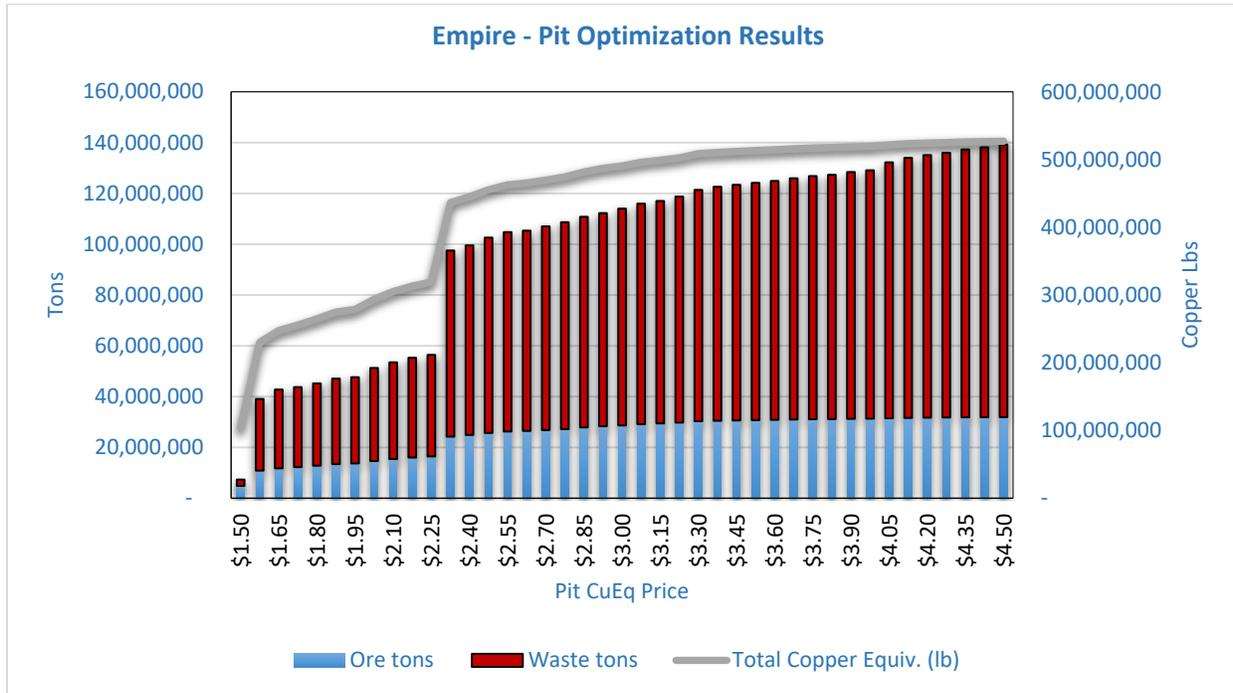
Figure 14-10 Pit Optimization Copper Sensitivity Chart
