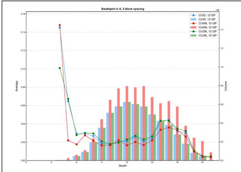
Figure E - 31 Swath Plot in the X Direction of Total Copper for the Granite Porphyry
