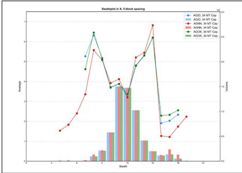
Figure E - 73 Swath Plot in the X Direction of Silver for the Magnetite Skarn
