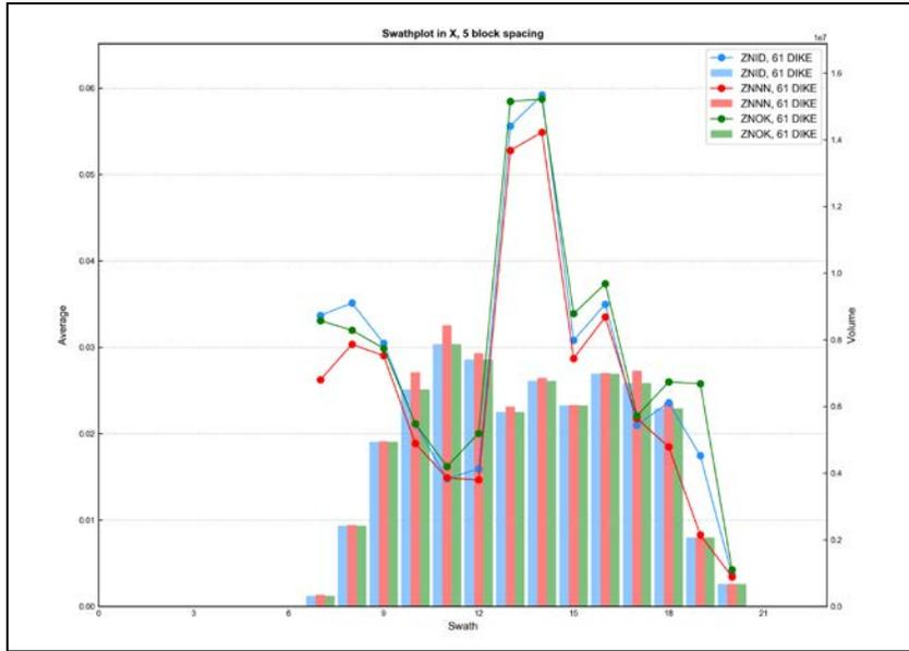
Figure E - 118 Swath Plot in the X Direction of Total Zinc for the Dikes
