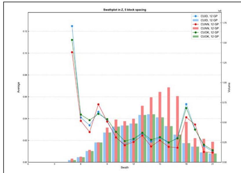
Figure E - 33 Swath Plot in the Z Direction of Total Copper for the Granite Porphyry
