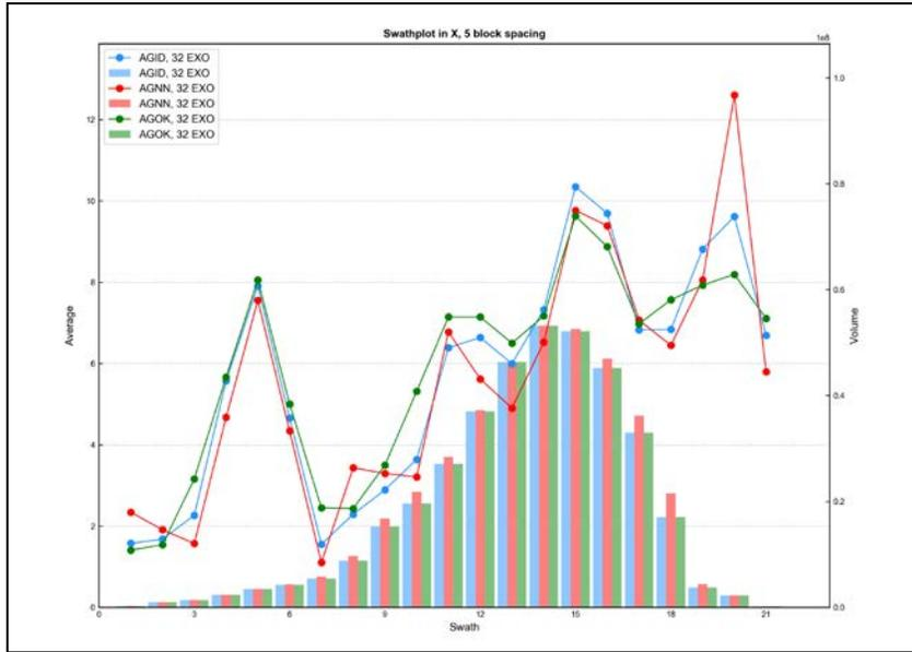
Figure E - 61 Swath Plot in the X Direction of Silver for the Pyroxene Skarn
