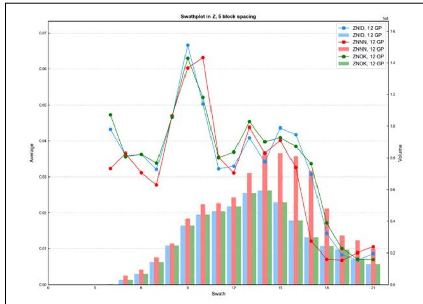
Figure E - 36 Swath Plot in the Z Direction of Total Zinc for the Granite Porphyry
