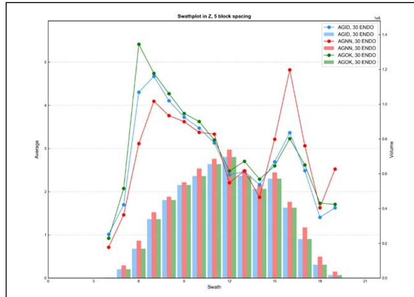
Figure E - 51 Swath Plot in the Z Direction of Silver for the Garnet Skarn
