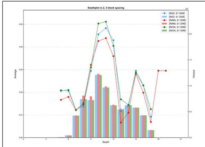
Figure E - 120 Swath Plot in the Z Direction of Total Copper for the Dikes
