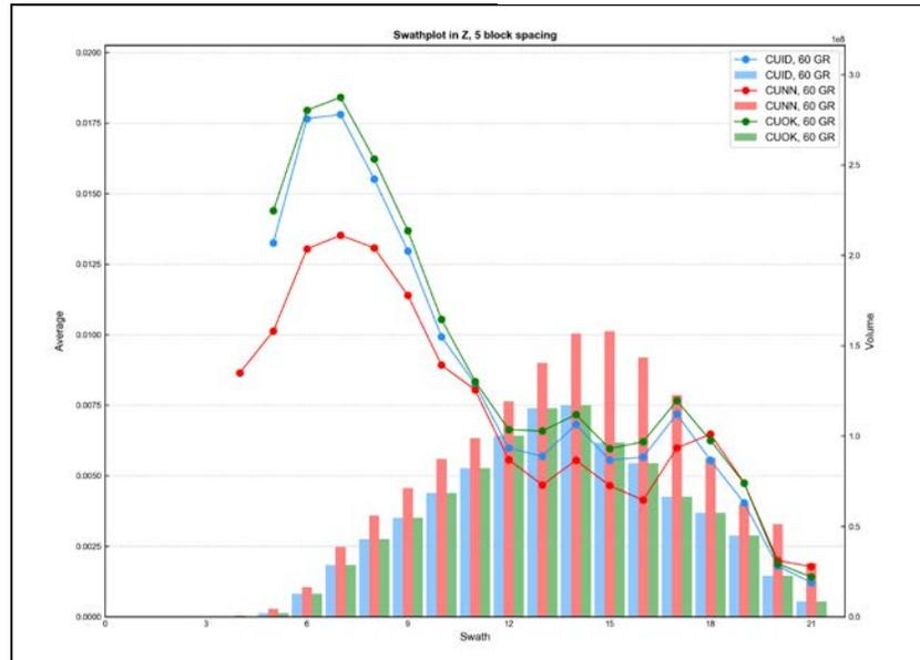
Figure E - 105 Swath Plot in the Z Direction of Total Copper for the Granite
