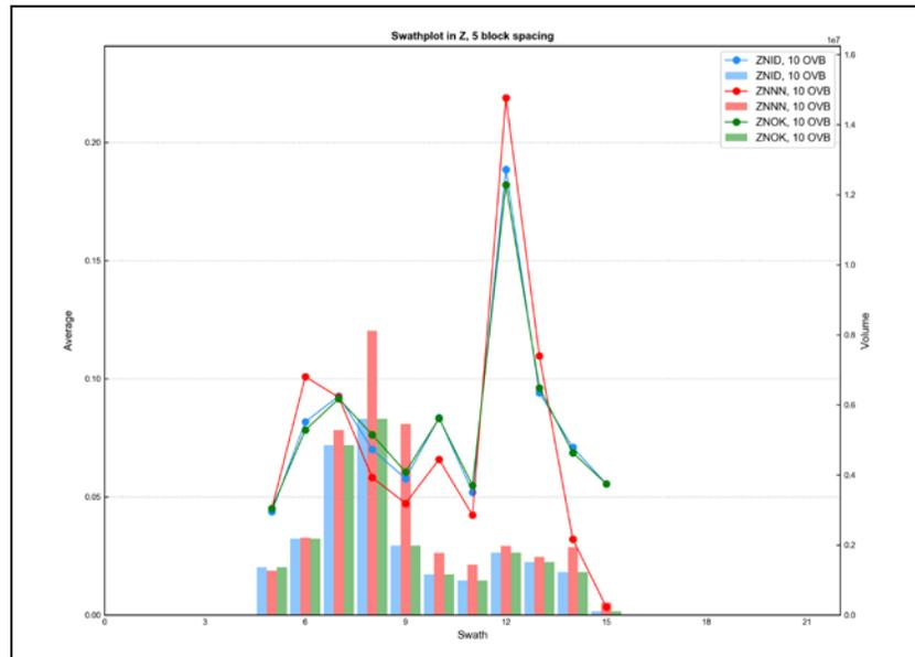
Figure E - 24 Swath Plot in the Z Direction of Total Zinc for the Overburden
