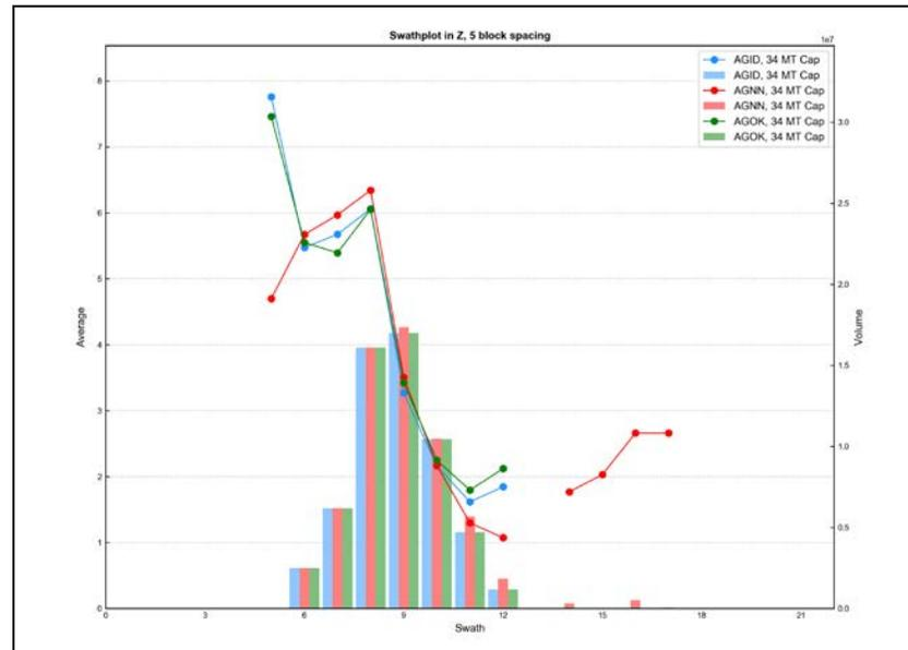
Figure E - 75 Swath Plot in the Z Direction of Silver for the Magnetite Skarn
