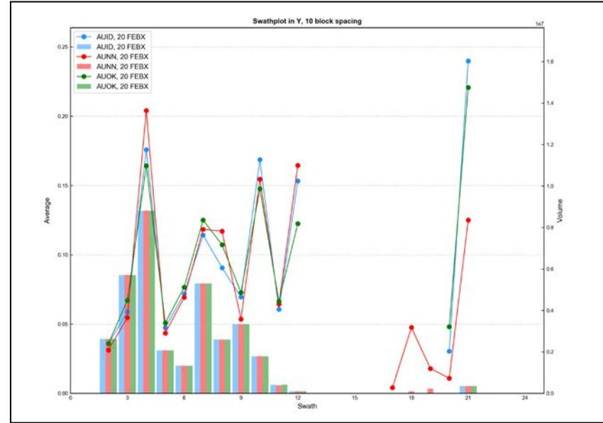
Figure E - 41 Swath Plot in the Y Direction of Gold for the Iron Oxide Breccia
