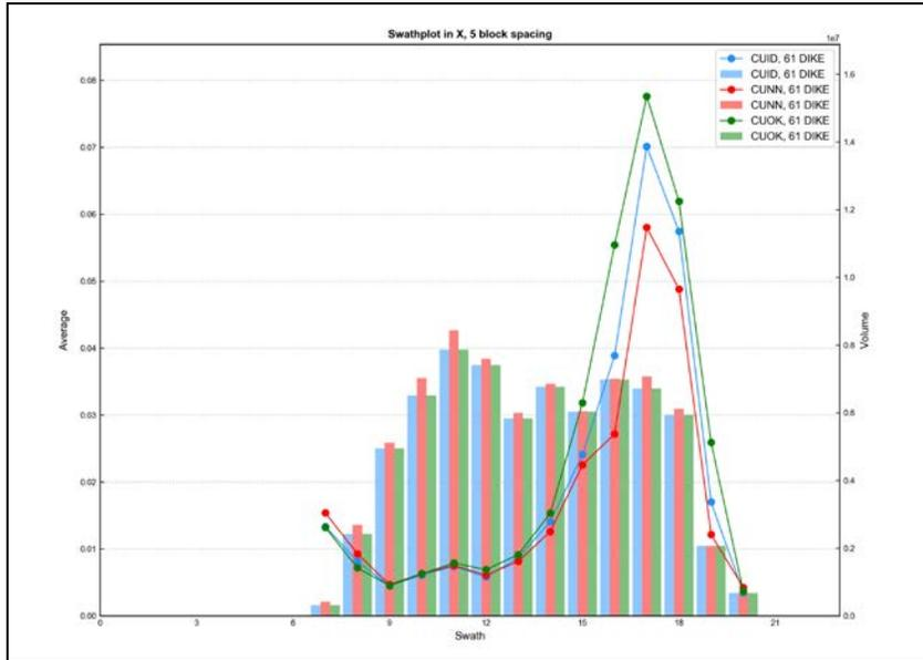
Figure E - 115 Swath Plot in the X Direction of Total Copper for the Dikes
