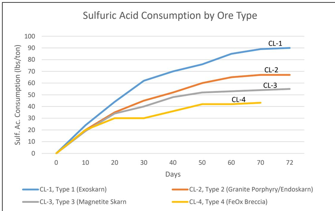
**Figure 13-2 Acid Consumption – Ore Type Column Test**
