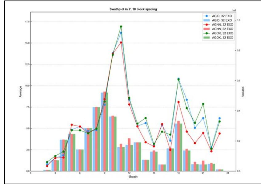
Figure E - 62 Swath Plot in the Y Direction of Silver for the Pyroxene Skarn
