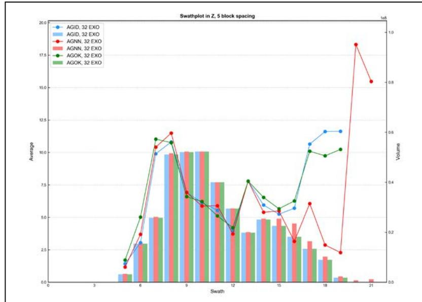
Figure E - 63 Swath Plot in the Z Direction of Silver for the Pyroxene Skarn
