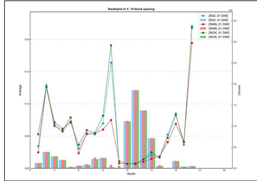
Figure E - 119 Swath Plot in the Y Direction of Total Copper for the Dikes
