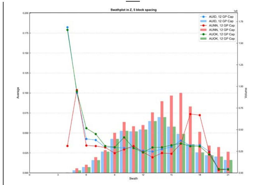
Figure E - 30 Swath Plot in the Z Direction of Gold for the Granite Porphyry
