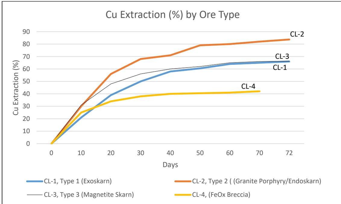
**Figure 13-1 Copper Extraction – Ore Type Column Tests**
