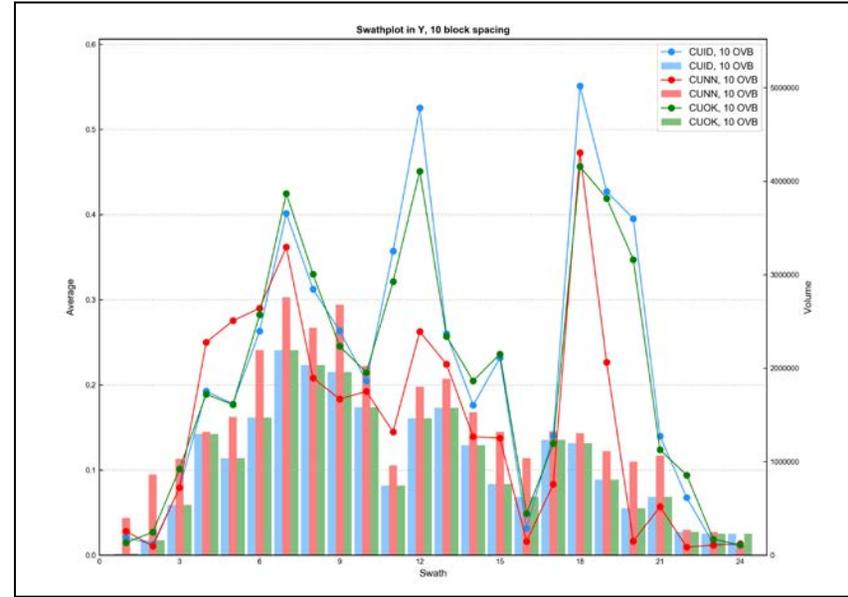
Figure E - 20 Swath Plot in the Y Direction of Total Copper for the Overburden
