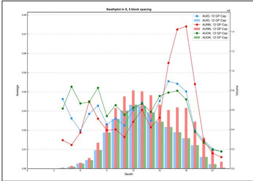
Figure E - 28 Swath Plot in the X Direction of Gold for the Granite Porphyry
