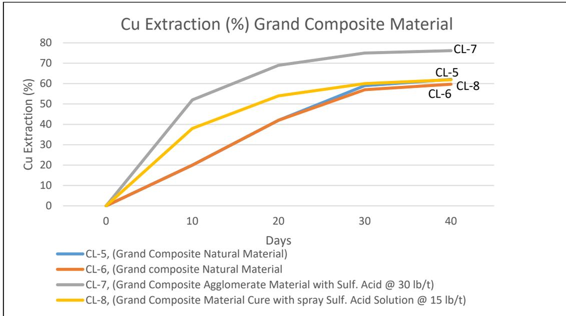
**Figure 13-3 Copper Extraction - Grand Composite Column Tests**
