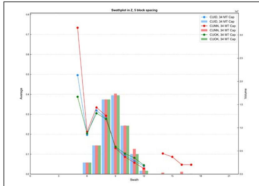
Figure E - 80 Swath Plot in the Z Direction of Total Copper for the Magnetite Skarn
