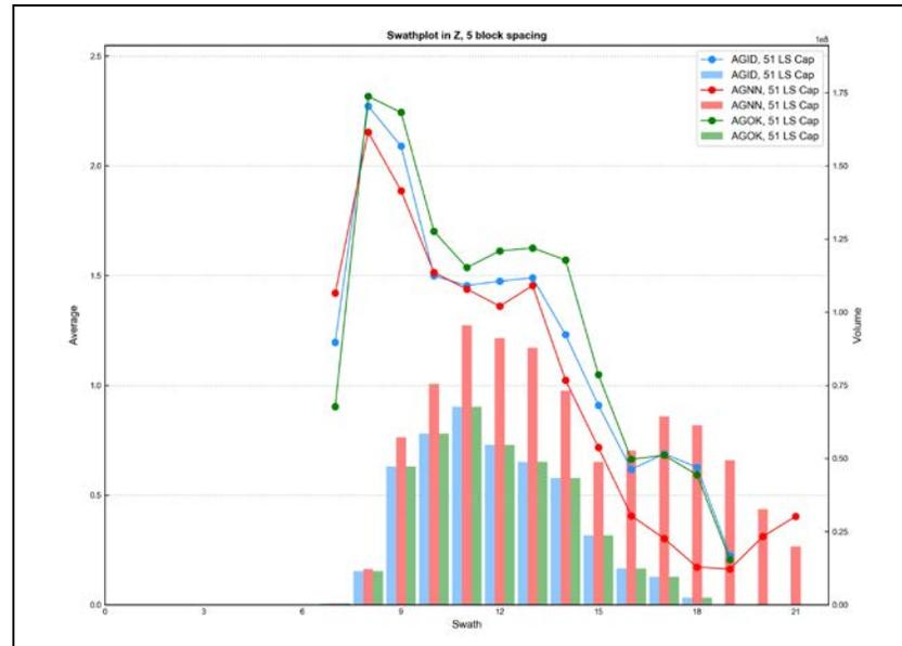
Figure E - 87 Swath Plot in the Z Direction of Silver for the Limestone
