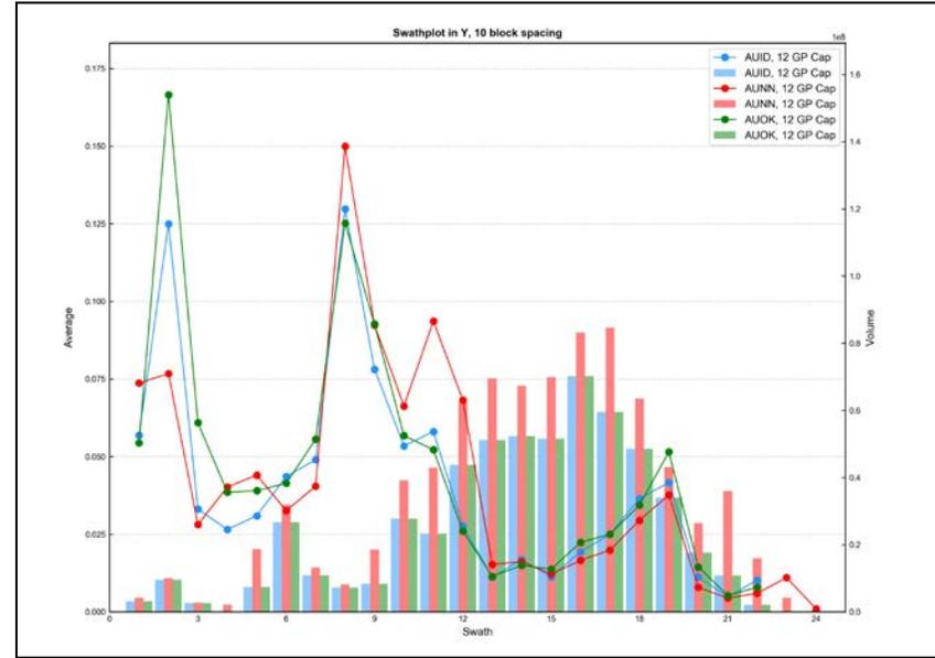
Figure E - 29 Swath Plot in the Y Direction of Gold for the Granite Porphyry
