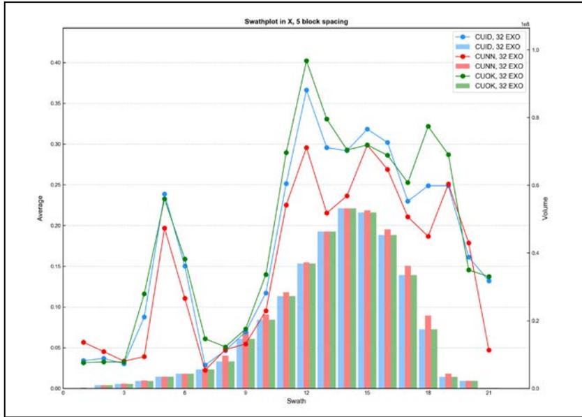
Figure E - 67 Swath Plot in the X Direction of Total Copper for the Pyroxene Skarn
