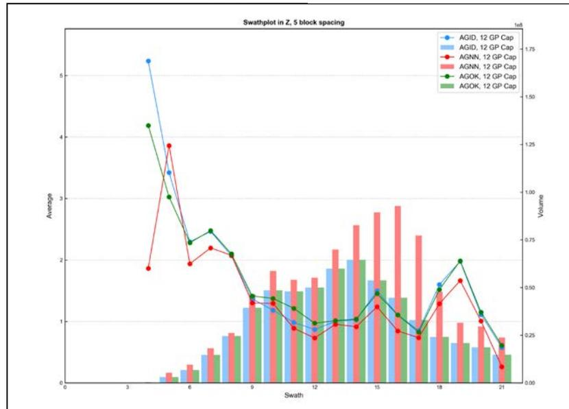
Figure E - 27 Swath Plot in the Z Direction of Silver for the Granite Porphyry
