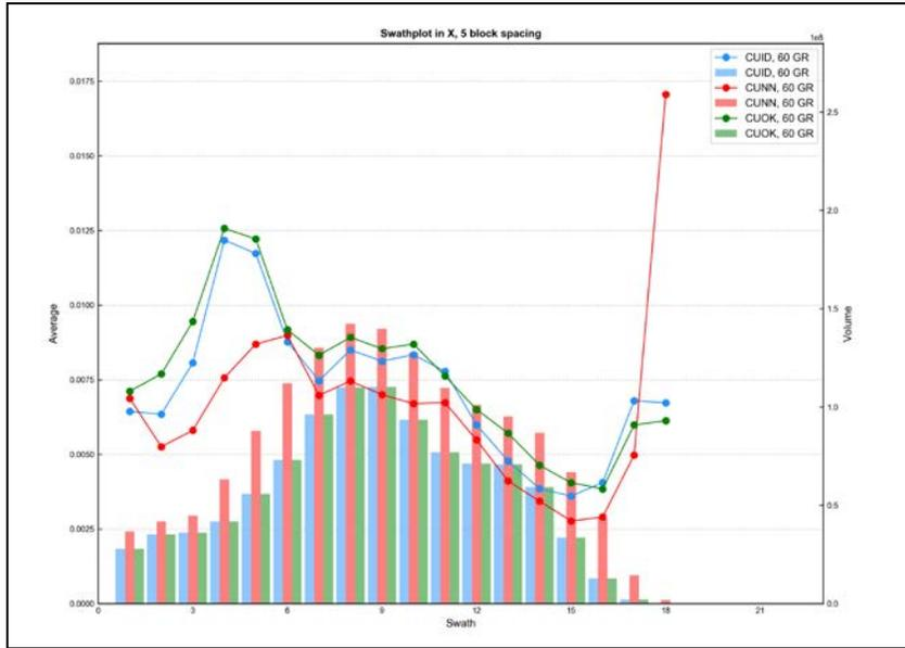
Figure E - 103 Swath Plot in the X Direction of Total Copper for the Granite
