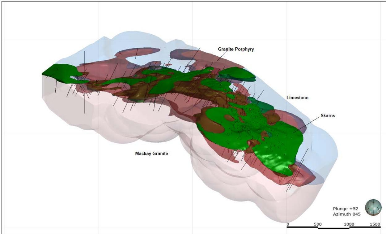
**Figure C - 1 Oblique View of the Broad Geologic Model.**
