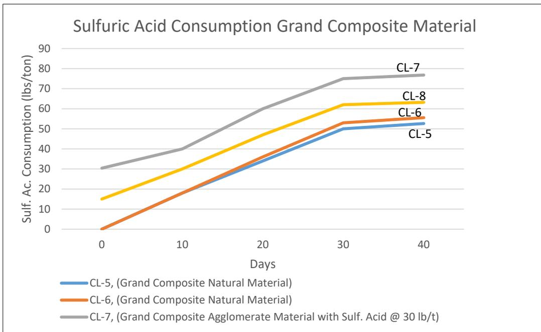
**Figure 13-4 Acid Consumption – Grand Composite Column Tests**
