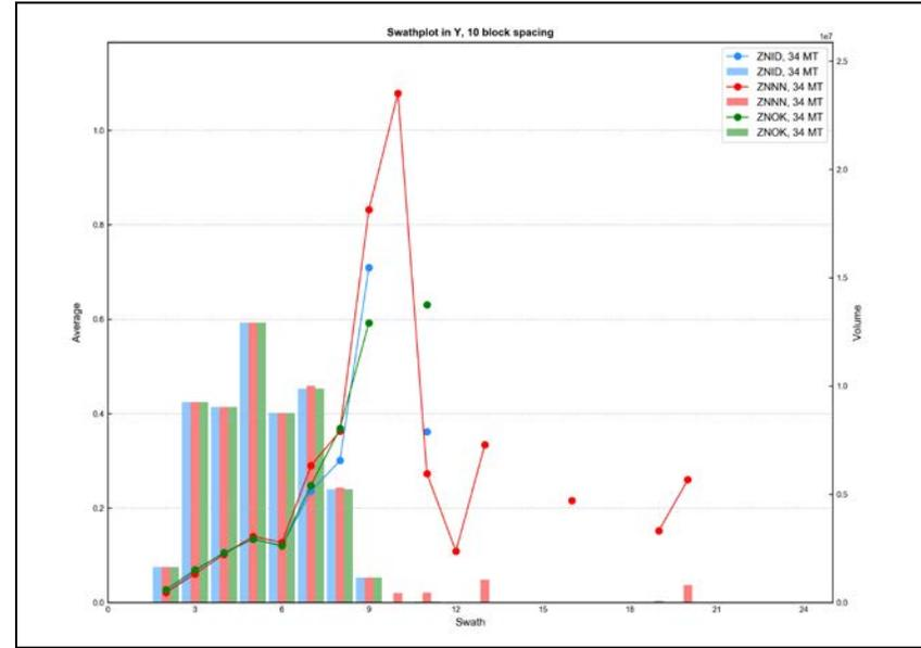
Figure E - 83 Swath Plot in the Y Direction of Total Zinc for the Magnetite Skarn
