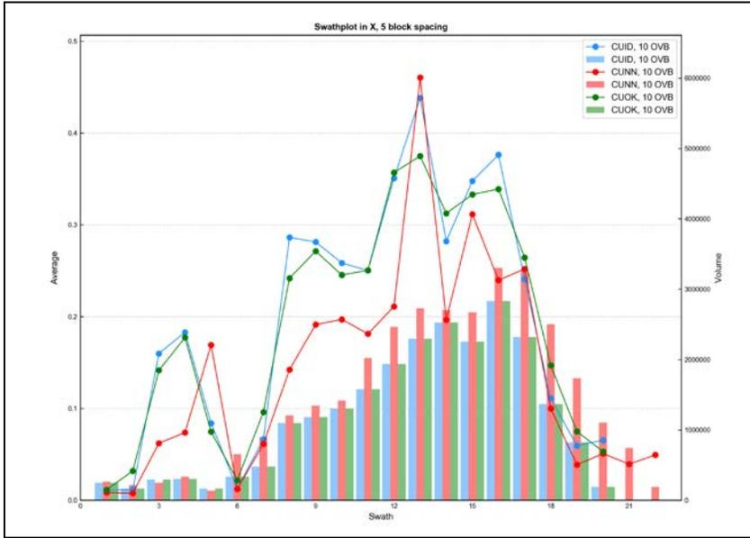
Figure E - 19 Swath Plot in the X Direction of Total Copper for the Overburden
