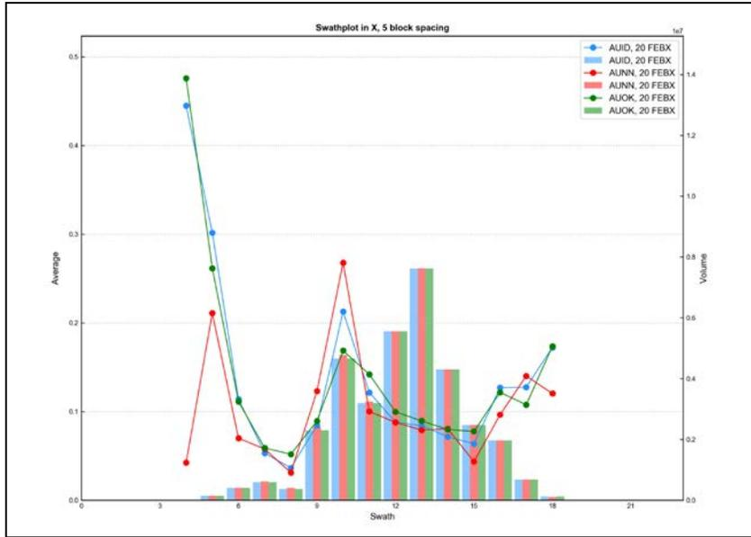
Figure E - 40 Swath Plot in the X Direction of Gold for the Iron Oxide Breccia
