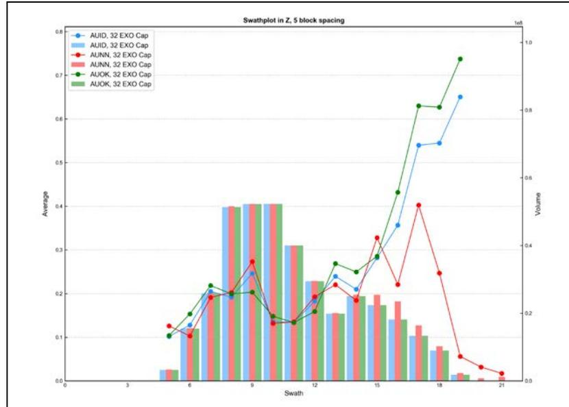
Figure E - 65 Swath Plot in the Z Direction of Gold for the Pyroxene Skarn
