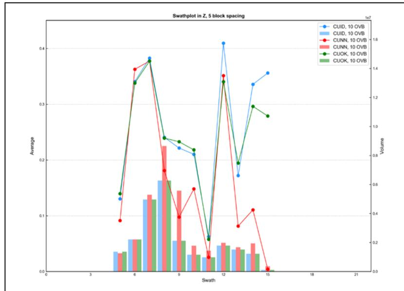
Figure E - 21 Swath Plot in the Z Direction of Total Copper for the Overburden
