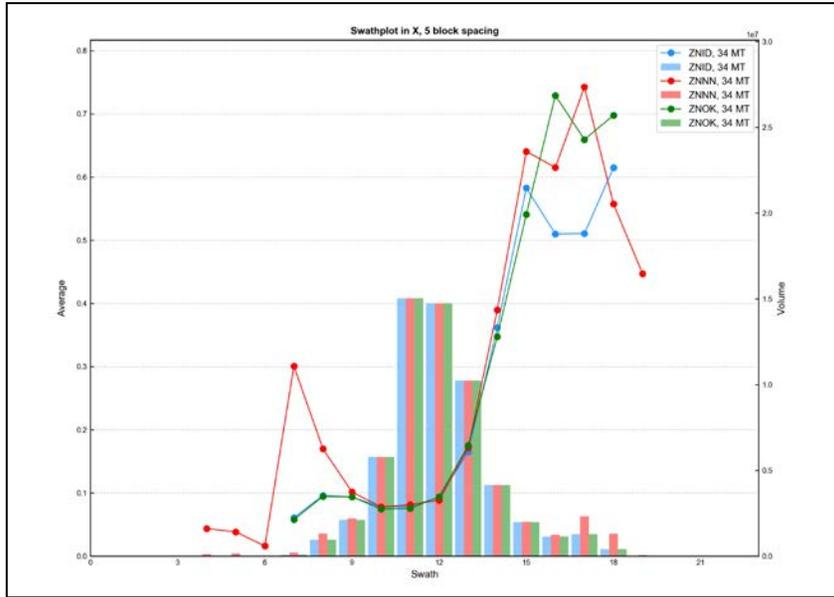
Figure E - 82 Swath Plot in the X Direction of Total Zinc for the Magnetite Skarn
