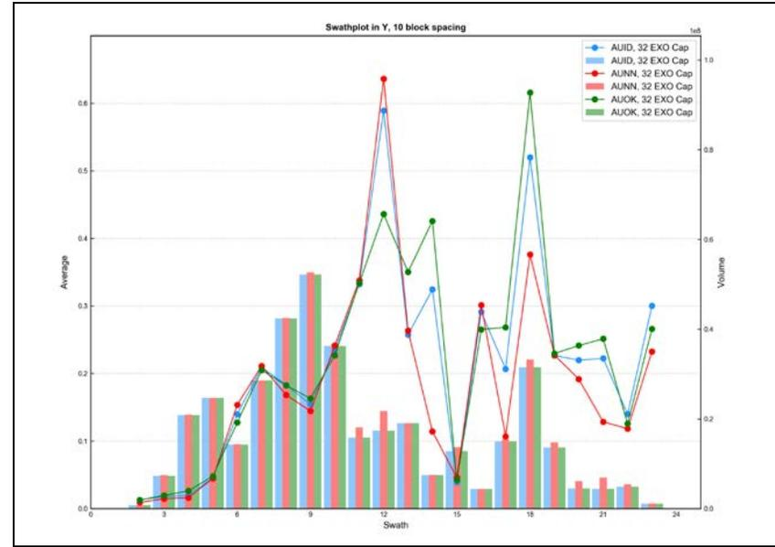
Figure E - 64 Swath Plot in the Y Direction of Gold for the Pyroxene Skarn
