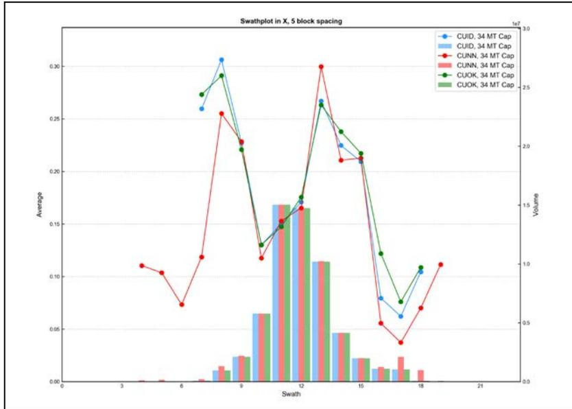
Figure E - 79 Swath Plot in the X Direction of Total Copper for the Magnetite Skarn
