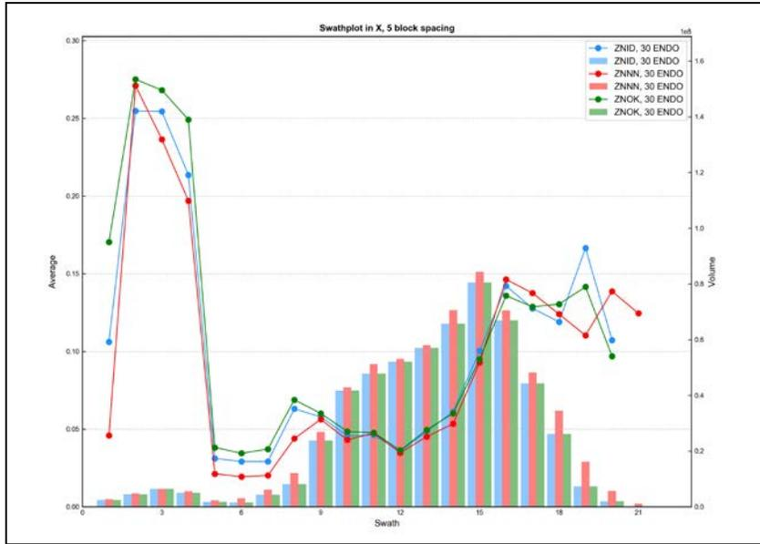
Figure E - 58 Swath Plot in the X Direction of Total Zinc for the Garnet Skarn
