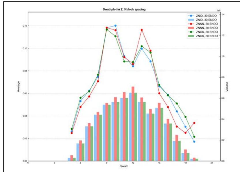
Figure E - 60 Swath Plot in the Z Direction of Total Zinc for the Garnet Skarn
