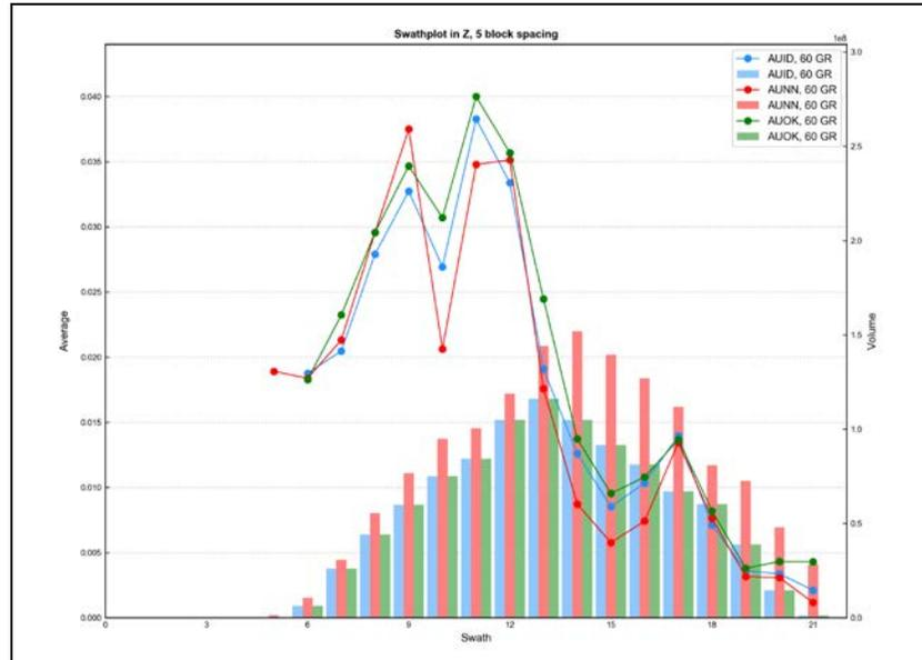
Figure E - 102 Swath Plot in the Z Direction of Gold for the Granite
