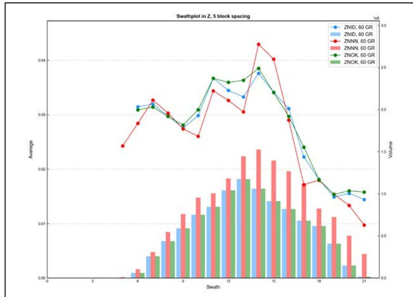
Figure E - 108 Swath Plot in the Z Direction of Total Zinc for the Granite
