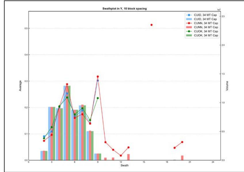
Figure E - 81 Swath Plot in the Y Direction of Total Copper for the Magnetite Skarn
