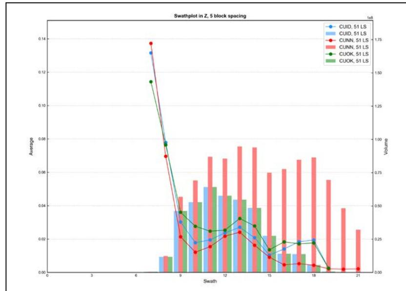
Figure E - 93 Swath Plot in the Z Direction of Total Copper for the Limestone
