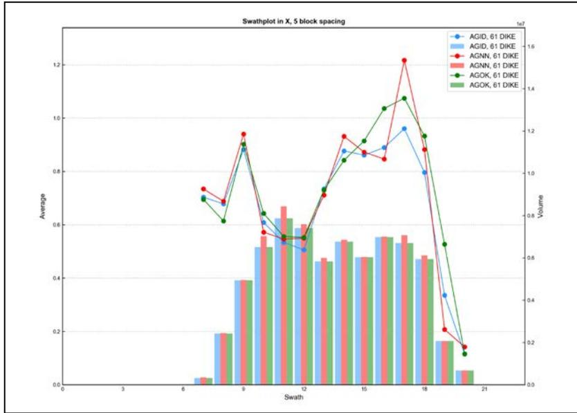
Figure E - 109 Swath Plot in the X Direction of Silver for the Dikes
