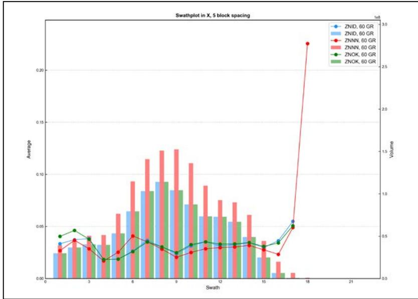
Figure E - 106 Swath Plot in the X Direction of Total Zinc for the Granite
