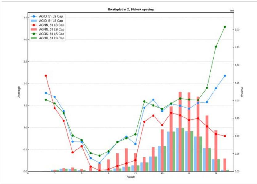
Figure E - 85 Swath Plot in the X Direction of Silver for the Limestone
