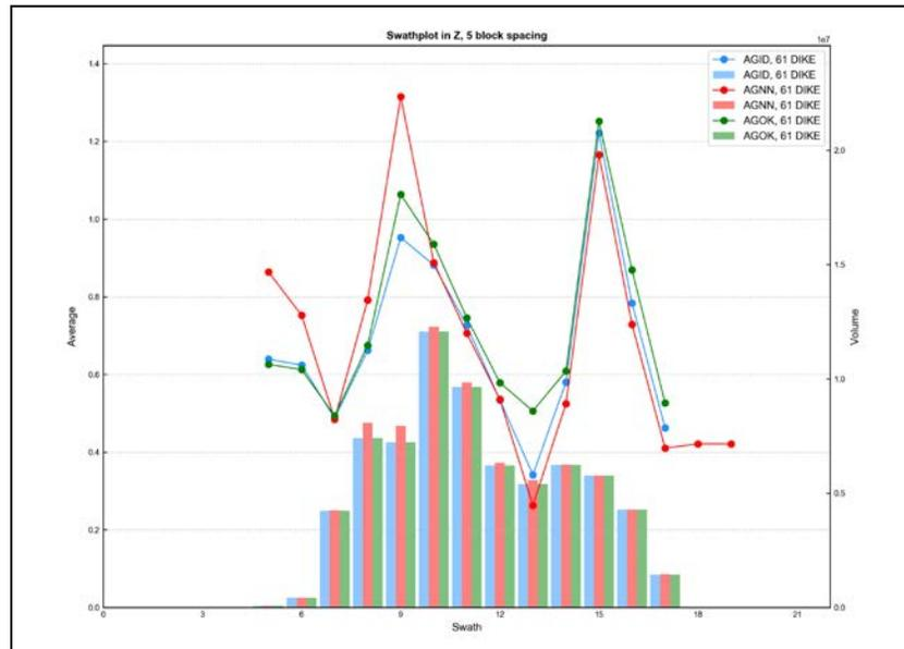
Figure E - 111 Swath Plot in the Z Direction of Silver for the Dikes
