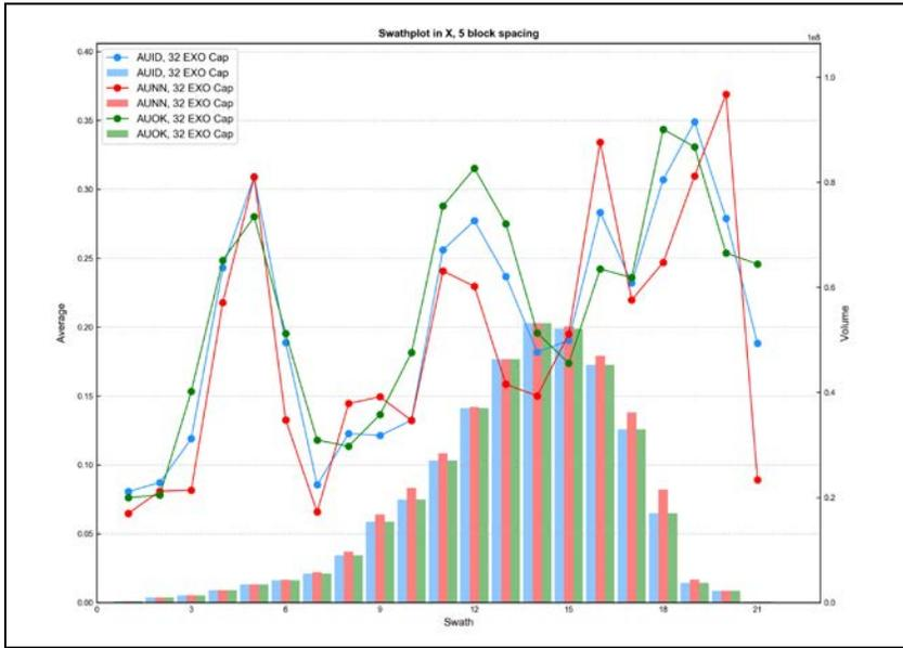
Figure E - 66 Swath Plot in the X Direction of Gold for the Pyroxene Skarn
